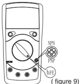
To measure transistor, connect the Meter as follows:
