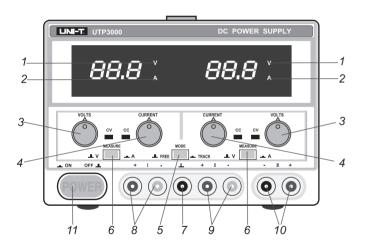
4) CURRENT: Adjust the output current at CC mode
