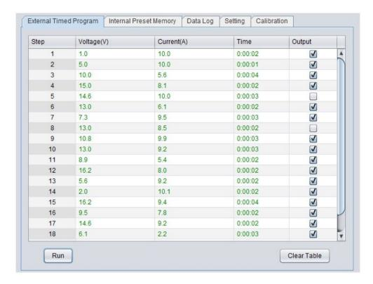
External Timed Program is completely controlled by PC, PC counts the time and changes voltage and current of power supply.
