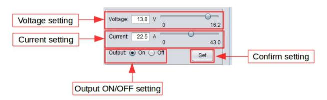
You can directly type the desired output voltage & output current and then click "Set" button to set the value. Or you can use slide bar to adjust the value.
