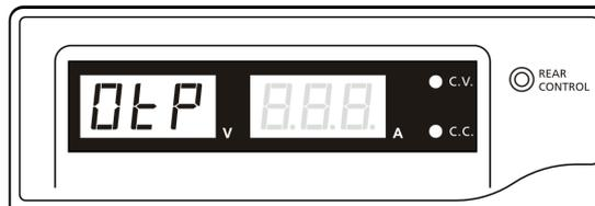
Check your load and output setting. Allow the unit to cool down for at least 30 minutes. Check if any of the ventilation is blocked, check enough clearance around power supply. Listen carefully for the short wind noise from the cooling fan when you turn on the unit again. If you cannot hear this routine self test wind noise on switch on, the fan is fault and do not use the power supply, contact your agent.
