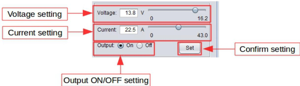
You can directly type the desired output voltage & output current and then click “Set” button to set the value. Or you can use slide bar to adjust the value.
