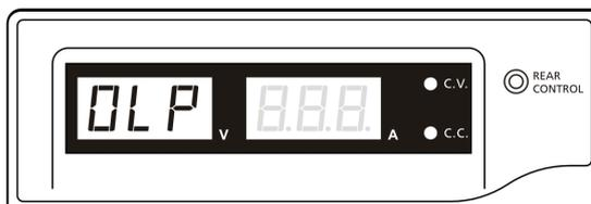
To reset this warning, switch off the unit and remove all loading. Switch the unit back on again and double check with caution. If this problem cannot be fixed, please contact and consult with your agent.
