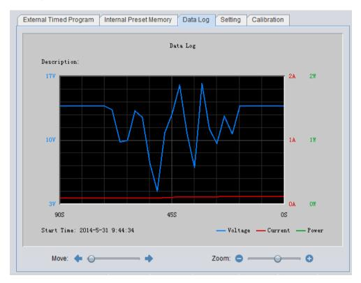
Data log window is used to display output Voltage, Current and Power against time in graphical view. You can move the diagram left and right by adjust "Move:" slide bar. You can zoom in/out the diagram by adjust "Zoom:" slide bar.
