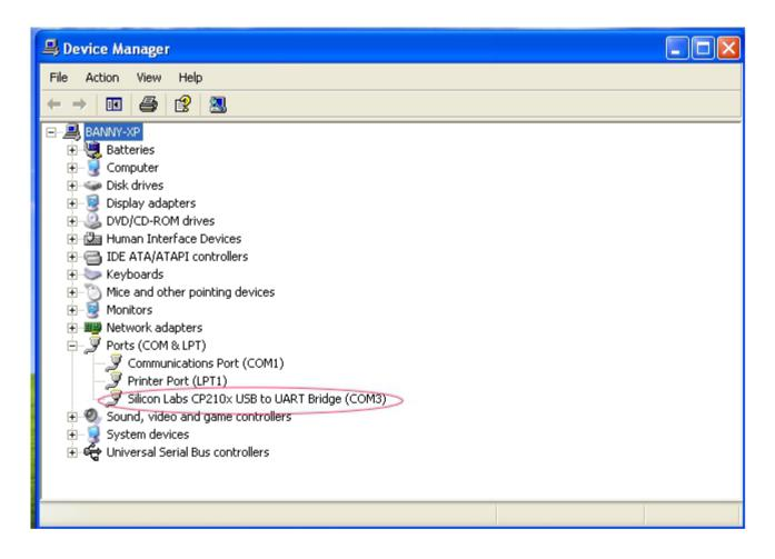
If the COM port does not come up, please check if the USB driver has been probably installed. The USB driver comes with HCS software CD. Make sure the CD has been load to computer first. Then it can program as stand COM port.
