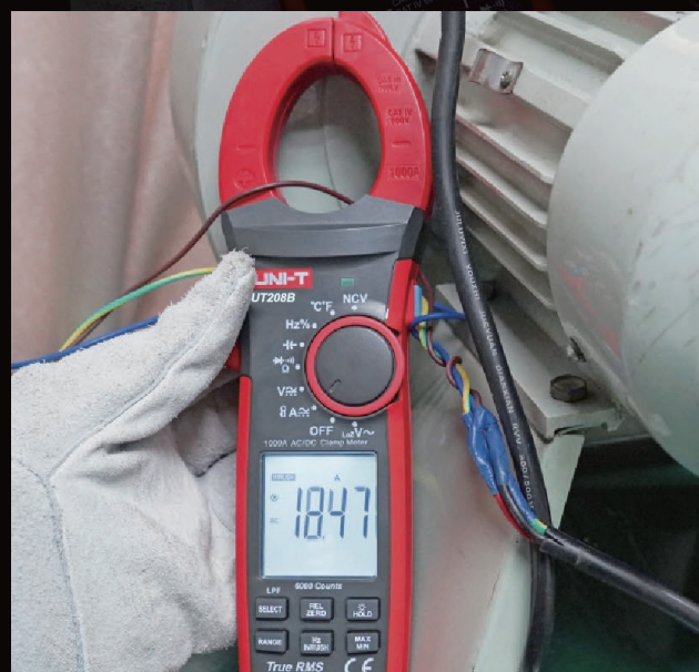
Inrush current capture (UT206B/207B/208B)
