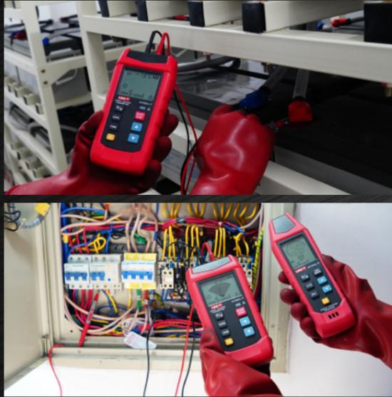
The measurement range is AC/DC 8~480V (AC frequency:50/60Hz), and the polarity can be identified.
