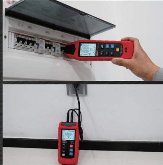
The locator can be used to find the correct RCD/GFCI or fuse location; No matter energized or none energized ones.
