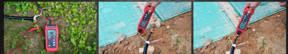
A specific wire can be quickly found in a multi-core cable, or multiple UT25CLT transmitters can be used at the same time with different codes.
