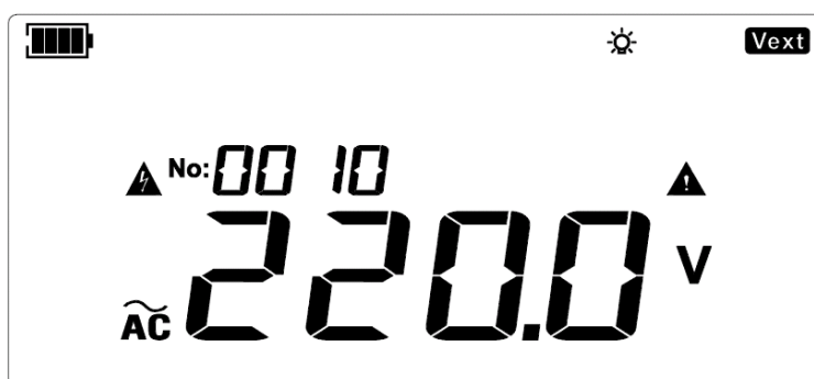
Figure 9.23 AC voltage measurement
