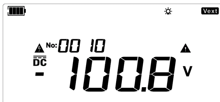
Figure 9.24 Negative DC voltage measurement
