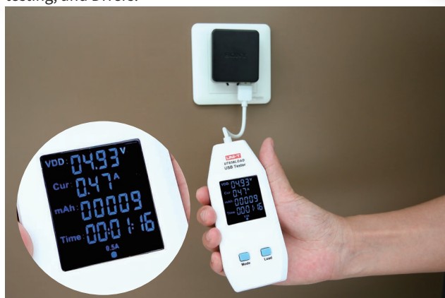
Tester with electronic load (UT658 LOAD)
