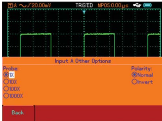
Figure 1-4 Adjusting the probe ratio
