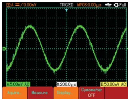
Figure 2-20 Waveform without average sampling
