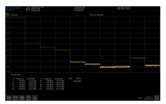
THD (total harmonic distortion) in output amplitude 0 dBm is less than 0.2%; Harmonic wave and stray in full frequency band are all less than -50 dBc.
