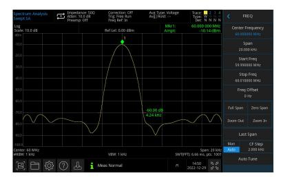
It has a stronger capability to resolve signals of adjacent unequal amplitudes.
