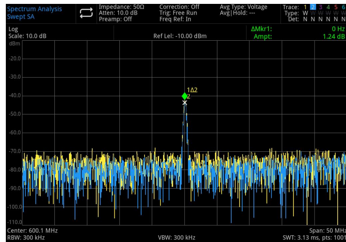
Figure 3-17 Component of Harmonic Distortion
